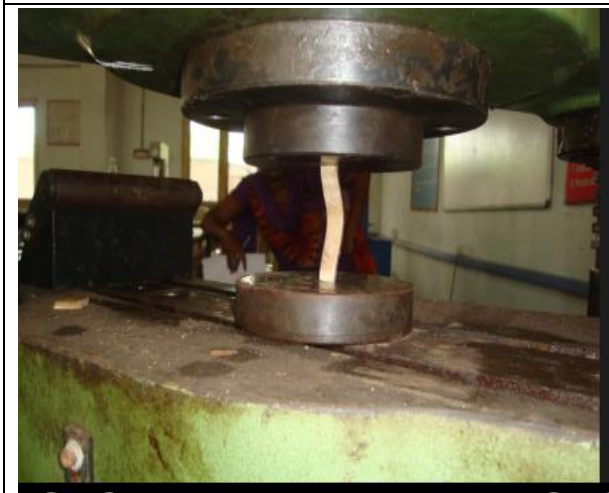
Fig.2.3 specimen during compression test
