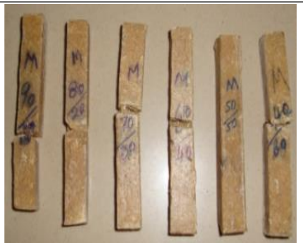
Fig.2.4 specimen after compression test
